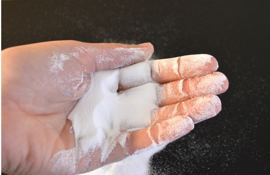
An example of plastic resin powder, a form of plastic raw material used in operations where a fine particle size is necessary for processing.
