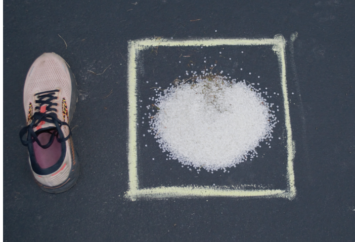
0.5 kg of clear plastic resin pellets inside a 1 ft 2 yellow square on asphalt beside a size 10 shoe.
