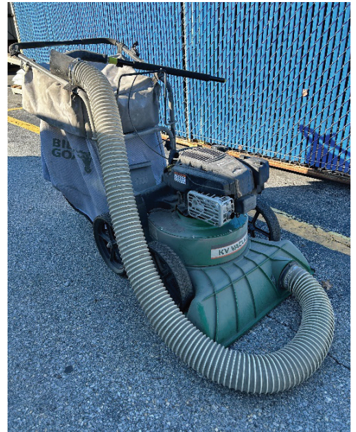
A portable vacuum used to clean spilled plastic resin at a transloading site.
