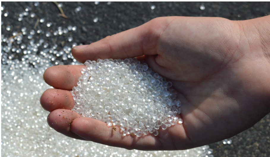
An example of plastic resin pellets, which are small granules used as the base material to create other plastic products. Preproduction plastic pellets vary in size but are typically between 1mm and 5mm.
